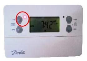
**Advance** moves the heating to the next setting. So if it is off at the moment, it turns on. If it is on at the moment, it turns off.
