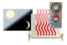
**24hrs** or **On** means the heating stays on all the time.
