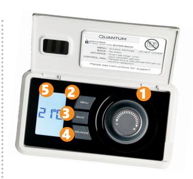
Press down the dial, and the display screen shows you the thermostat target temperature and timer mode.
