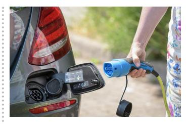
Some EVs can be used to power your home, just like a domestic battery. For this to be possible, the EV and the EV charger will need to be bi-directional charging compatible.
