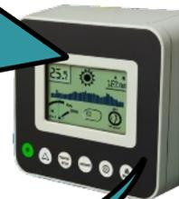
The **meter** measures how much electricity your panels are making.
